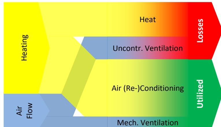
Fig 8. Breakdown of utilization and losses of active processes observed in tobacco curing
