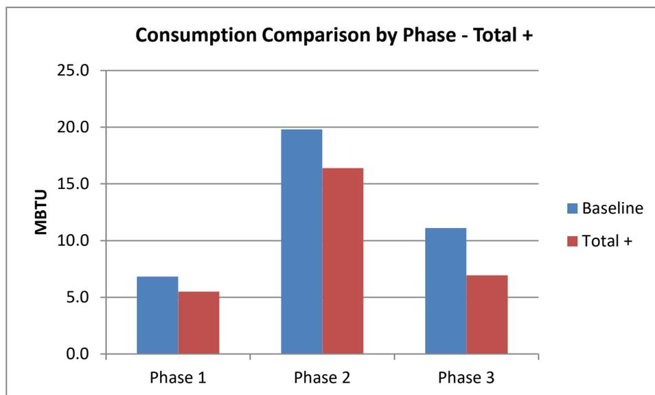
Fig 32. Comparison of energy consumption of retrofit scenario “Total +” and baseline scenario by curing phase
