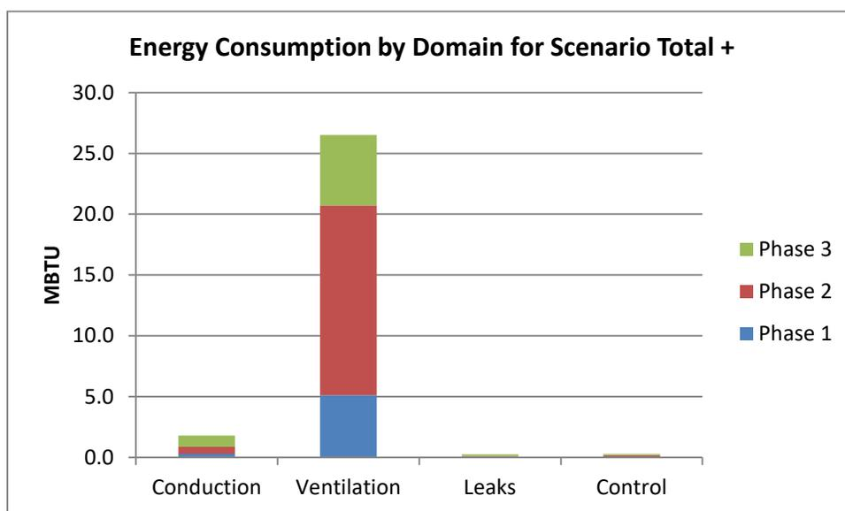
Fig 30. Total energy consumption after retrofit scenario "Control +" has been applied. Over-ventilation has been reduced to a minimum.
