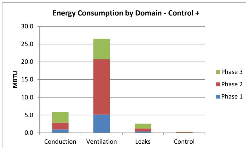
Fig 26. Total energy consumption after retrofit scenario “Control +” has been applied. Over-ventilation has been reduced to a minimum.
