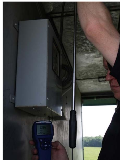
Fig 19. Velocity in the return plenum leaving the curing compartment
